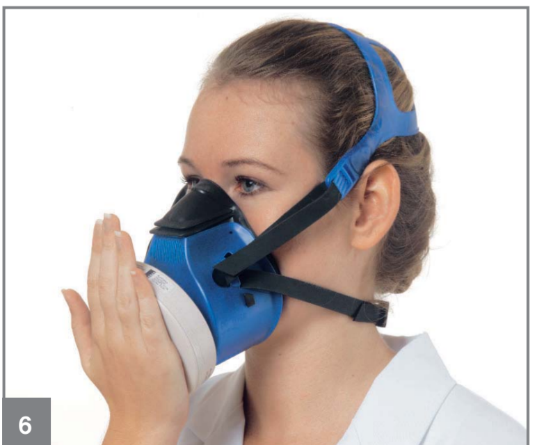
6 Seal the respiratory filter with your hand and breathe in until a negative pressure (suction) is generated. Hold your breath for a moment. The negative pressure should be maintained. If not, readjust the face piece and adjust the straps or use a different size of mask. Repeat test until a successful seal check is met.
